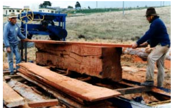
Laidlaw Bushmill. Horizontal bandsaw.
